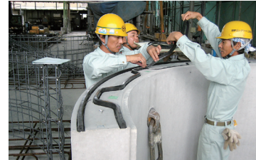
Application of TS seal tape for joining drop-off manholes
