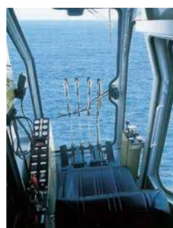
Operating seat for LGP series (with 4 levers)
