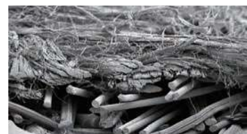
Cross section of NA superfine acrylic fiber nonwoven fabric
