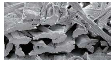
Cross section of ordinary rayon nonwoven fabric
