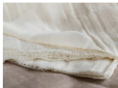
Cross section of 8-layer gauze blanket
